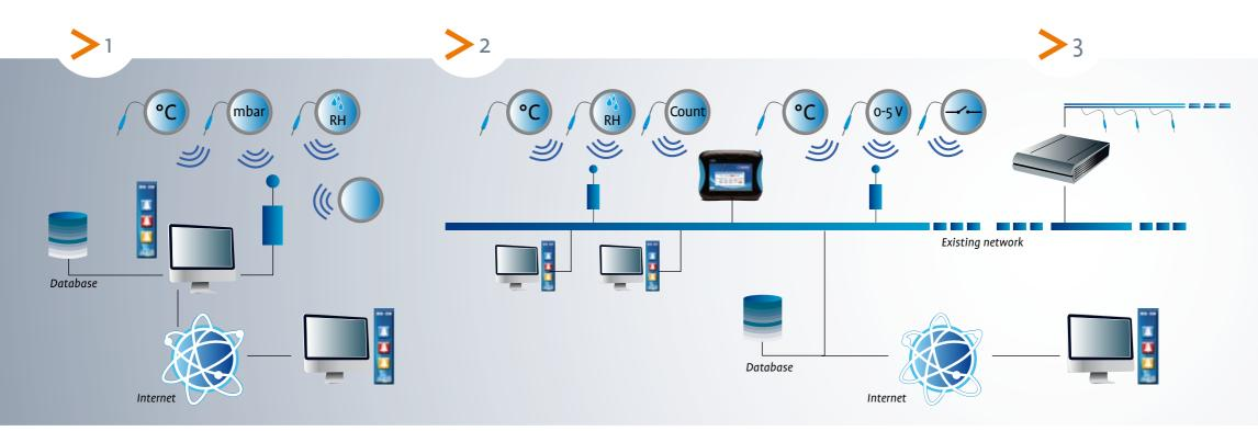
1/ Radio frequency transmission. Installation of the eviSENSE<sup>®</sup> software with its database on a PC connected to the radio receiver (network installation possible). Access possible via Internet.
