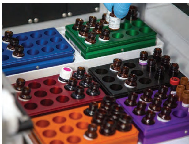
PS-10 reagent blocks hold up to 90 antibody reagent vials of different sizes
